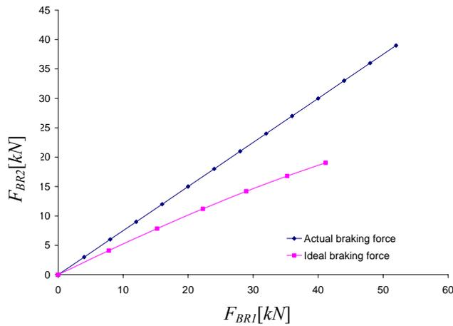
Figure 6: Relation of brake force distribution between twin and rear axles
