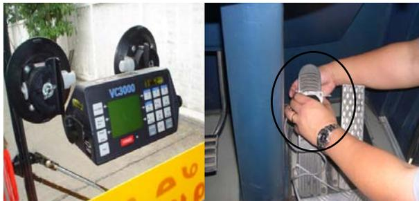
Figure 3: (a) Installation of VC3000 at the windshield (b) the foot brake sensor
