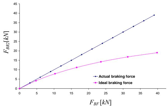
Figure 5: Relation of brake force distribution between front and rear axles
