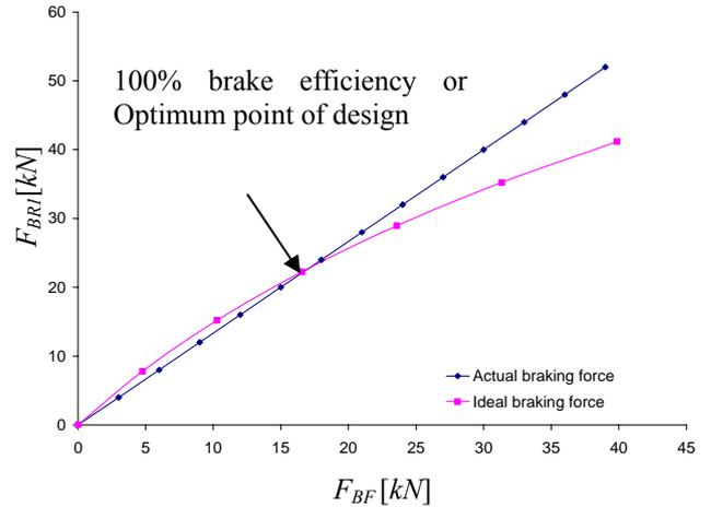
Figure 4: Relation of brake force distribution between front and twin axles
