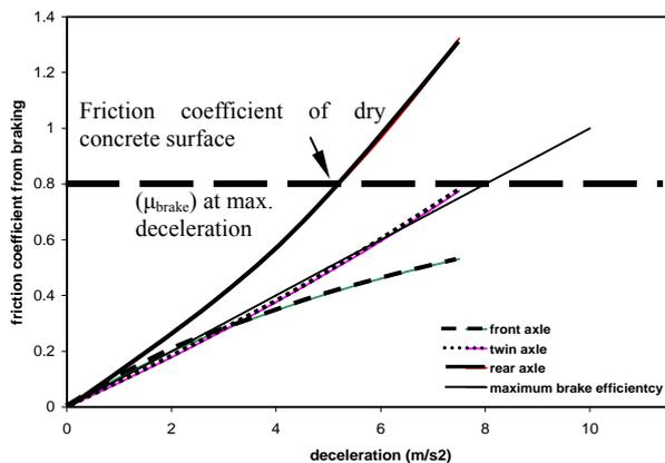
Figure 8: Friction coefficient from braking at various decelerations
