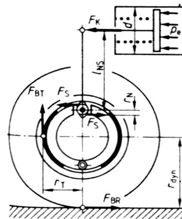
Figure 1: Drum and shoe layout
