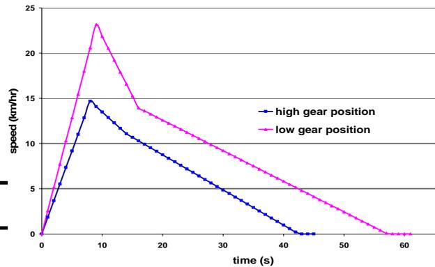
Figure 7: Speed behaviour during engine brake tests
