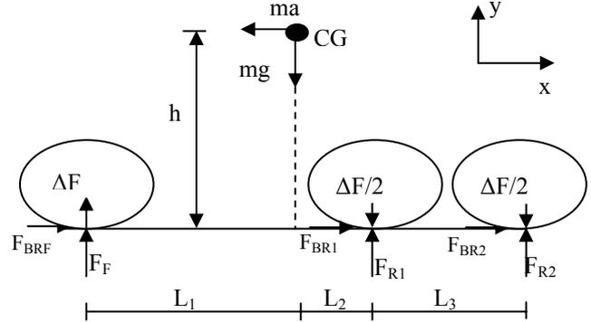
Figure 2: Free body diagram [FBD] of bus
