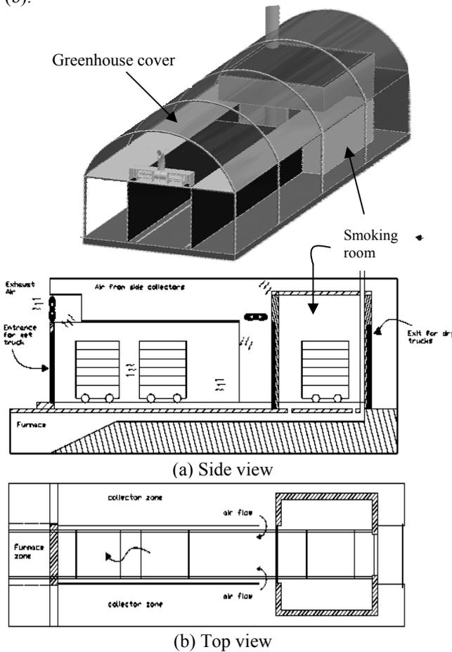
Fig. 3. Conceptual design initially of the greenhouse drying.
