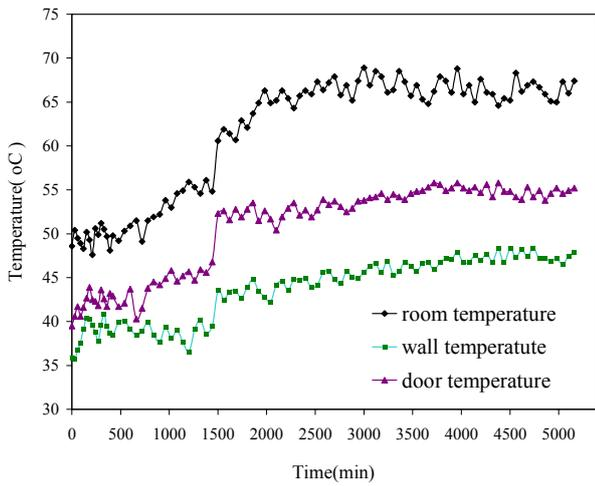
Fig. 2 room, wall and door temperature of smoking room (old system)
