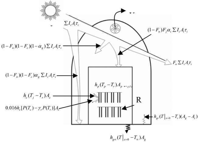
Fig. 4 Principle of solar rubber sheet drying under greenhouse forced convection
