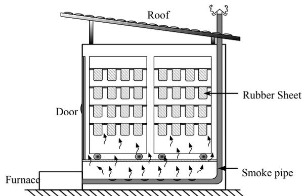
Fig. 1 Natural rubber sheet smoking room (old system).
