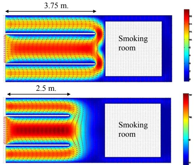
Fig. 5. Air flow character of greenhouse at length of portion for keeping pushcart
