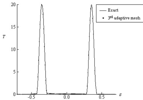
Fig. 11. Comparison of the exact and the predicted solutions for a 4-step gradient cones in a square region problem.
