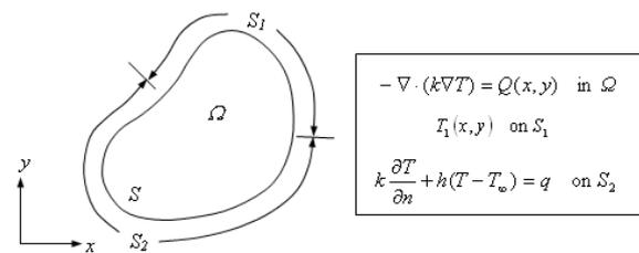
Fig. 1. Two-dimensional domain and boundary conditions for problem governed by energy equation
