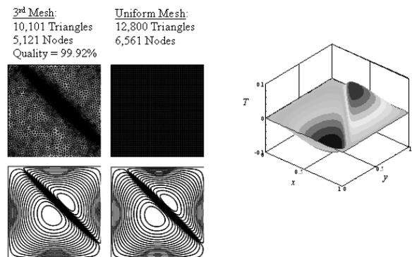
Fig. 7. Uniform and adaptive meshes with their solution contours for a highly heat source along diagonal line problem.
