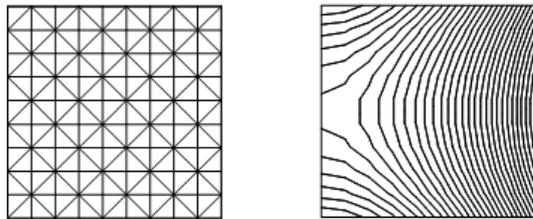
Fig. 4. Problem statement of the Laplace equation with Dirichlet boundary conditions.
