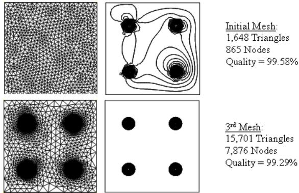
Fig. 10. Initial and adaptive meshes with their solution contours for a 4-step gradient cones in a square region problem.
