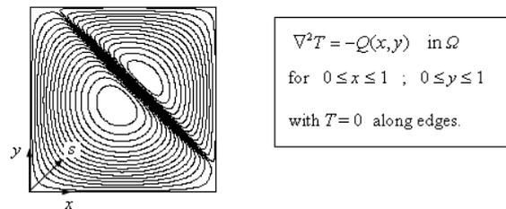
Fig. 6. Governing equation, boundary conditions, and solution contours for a highly heat source along diagonal line problem.
