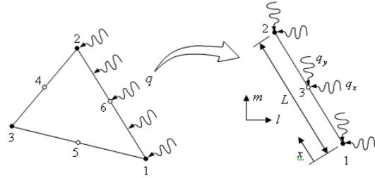
Fig. 2. Discretization of flux vector  $q$  into the actual nodes and the nodeless variable on a typical element edge.
