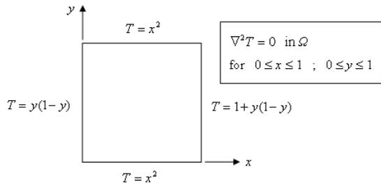
Fig. 3. Problem statement of the Laplace equation with Dirichlet boundary conditions.
