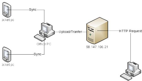
Fig. 2 Architecture of the proposed system
