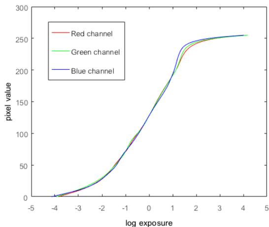
Fig. 2 The camera response curve of DSLR camera
