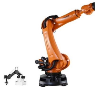
Figure 1. a budget robotic arm eg., DOBOT magician (left) and an industrial robotic arm (right) e.g., KUKA.
